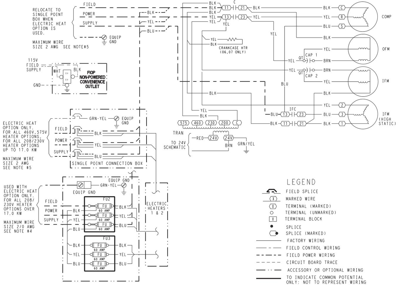
**Fig. 17 - 1-Stage Cooling Typical Power Diagram**
