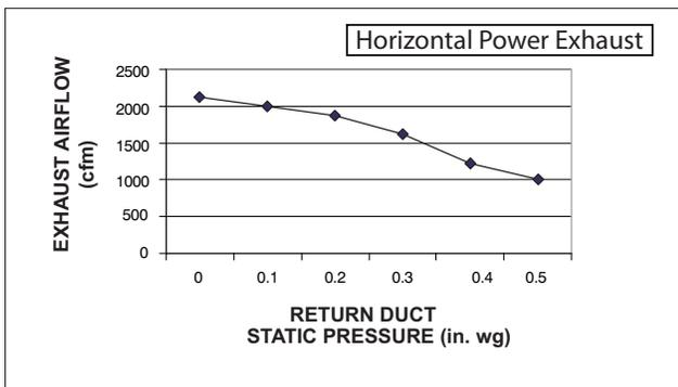
**Fig. 12 - Horizontal Power Exhaust Performance**
