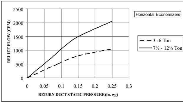
**Fig. 9 - Barometric Relief Flow Capacity**
